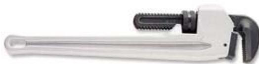
The upper jaw is forged in heat-treated steel, equipped with 2 springs ensuring efficient self-tightening on the pipe and allowing ratchet-like action. Double high-frequency hardened teeth. Lightweight, very easy to handle. Replaceable lower jaw.
